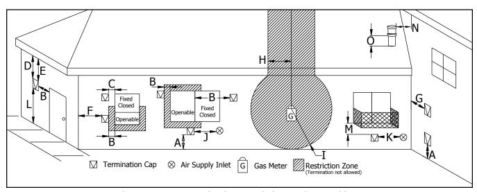
Figure 19. Vent Termination Restrictions, refer to Table 2.
